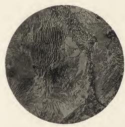
Fig. 22. Iron containing 1.7 per cent. P. and 0.71 per cent. C. Shows phosphide eutectic surrounding the grains of pearlite and ferrite.
